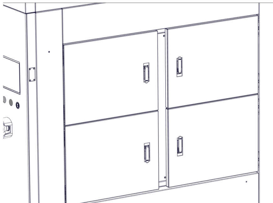
Figure 3.8 Four independent filament chambers
